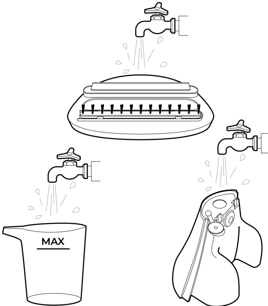
Figure 19 – Cleaning the water tank and accessories
